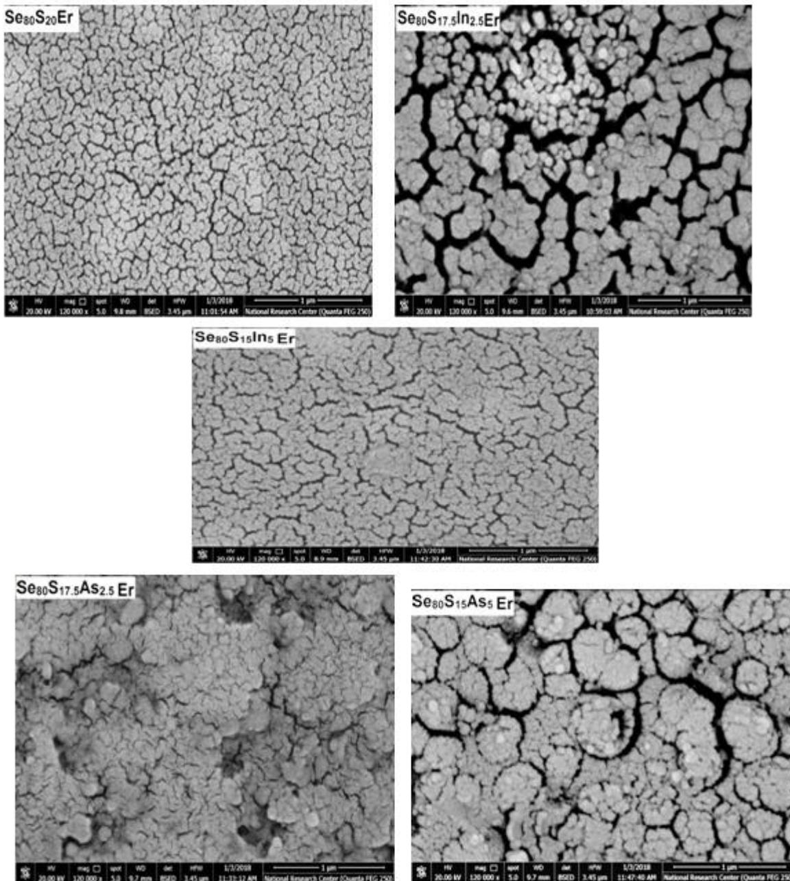
Fig [5] scanning electron micrograph image of chalcogenide system  $Se_{80}S_{20-x}B_x$  where ( $x=0,2.5,5$  and  $B=In$  or  $As$ ) thin films covered with Er layer
