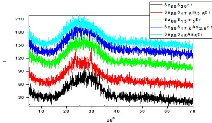
Fig [3] X-ray diffraction patterns of system  $Se_{80}S_{20-x}B_x$  where ( $x=0,2.5,5$  and  $B=In$  or  $As$ ) thin film after covering Er layer.
