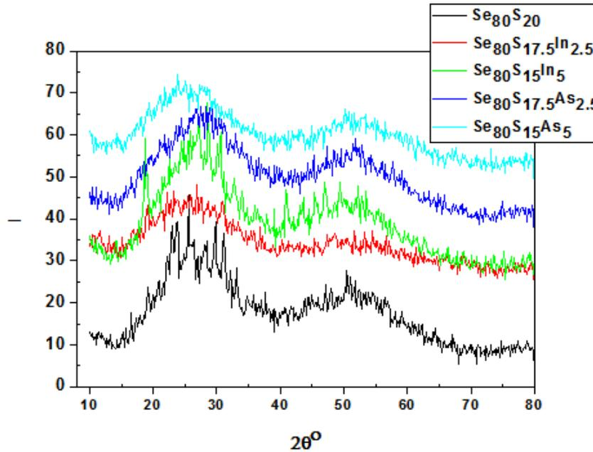
Fig [1] X-ray diffraction patterns of system  $Se_{80}S_{20-x}B_x$  where ( $x=0,2.5,5$  and  $B=In$  or  $AS$ ) as bulk samples .
