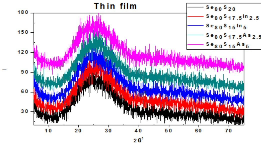
Fig [2] X-ray diffraction patterns of system  $Se_{80}S_{20-x}B_x$  where ( $x=0,2.5,5$  and  $B=In$  or  $AS$ ) thin film deposited on a glass substrate.
