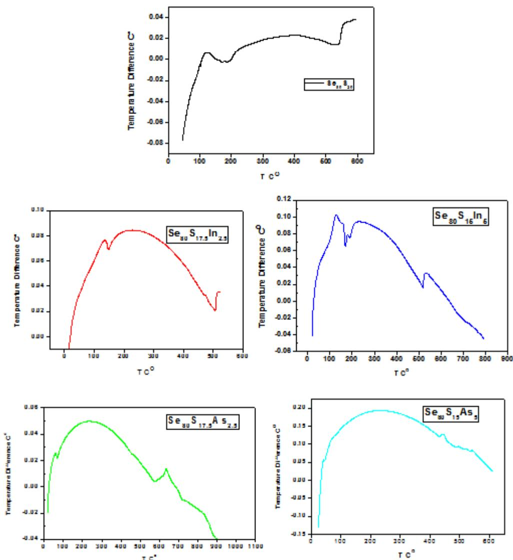
Fig [6] DTA thermograms of chalcogenide system  $Se_{80}S_{20-x}B_x$  where  $(x=0,2.5,5$  and  $B=In$  or  $As$ ).
