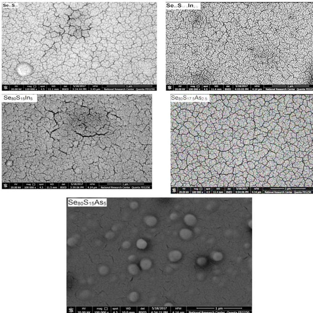
Fig [4] scanning electron micrograph image of chalcogenide system  $Se_{80}S_{20-x}B_x$  where ( $x=0,2.5,5$  and  $B=In$  or  $As$ ) thin film.
